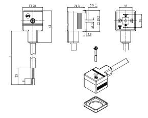
Molded Cable DIN Valve Connectors
