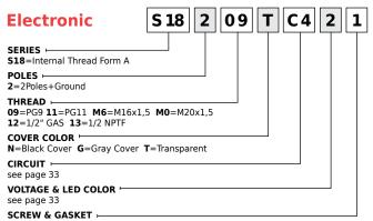
1=Profile NBR Gasket & Screw, 2=Flat NBR Gasket & Screw 3=White Silicone Profile Gasket & Screw, 4=White Silicone Flat Gasket & Screw
