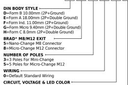
**A**=Circuit S0 24V and Yellow LED **B**=Circuit C4 24V and Yellow LED
