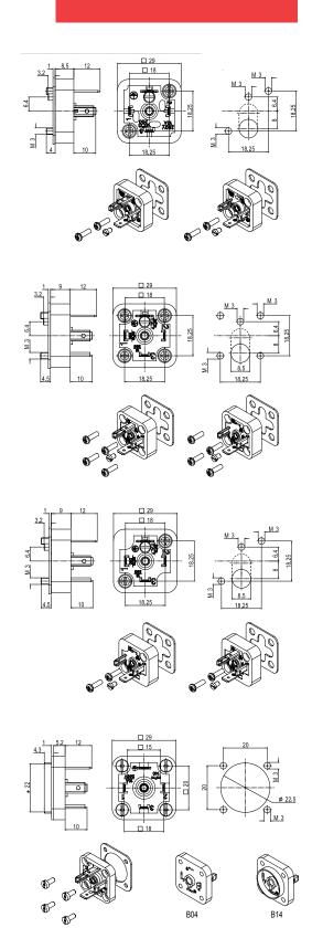
DIN Bases are provided in kit with fixing screw and gasket where required. The range covers the most important and common applications.
